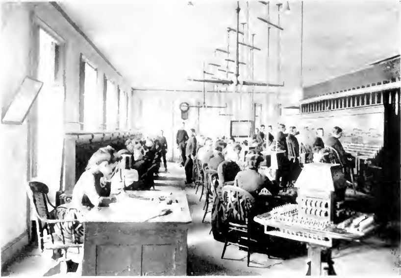
A NEW YORK CITY CENTRAL OFFICE IN THE '80S, SHOWING "BEEHIVE" AS WELL AS EARLY DESK TYPE SWITCHBOARDS, AND BOTH YOUNG WOMEN AND BOY OPERATORS
